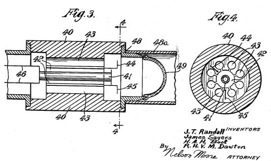
MEANS FOR TRANSFERRING POWER TO AND FROM MAGNETRONS
